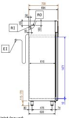
FΙ Electrical inlet (power) RI Refrigerant Inlet Refrigerant Outlet
